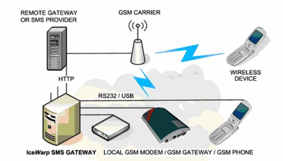
2N Voiceblue GSM Gateway. An example of a hardware gateway which can communicate over USB as a locally connected modem or over Ethernet as an HTTP remote gateway.
